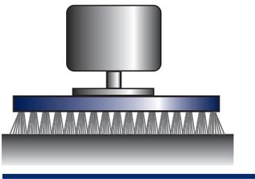
**Disc brushes** provide aggressive scrubbing on smooth floors and can adjust to dips in the floor, providing a constant downward pressure.
