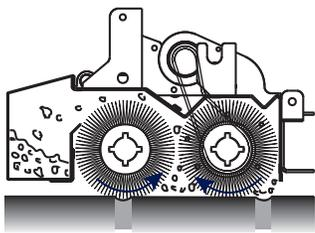
**Cylindrical brushes** pick up light debris on grouted floors and eliminate the need for pre-sweeping prior to scrubbing.
